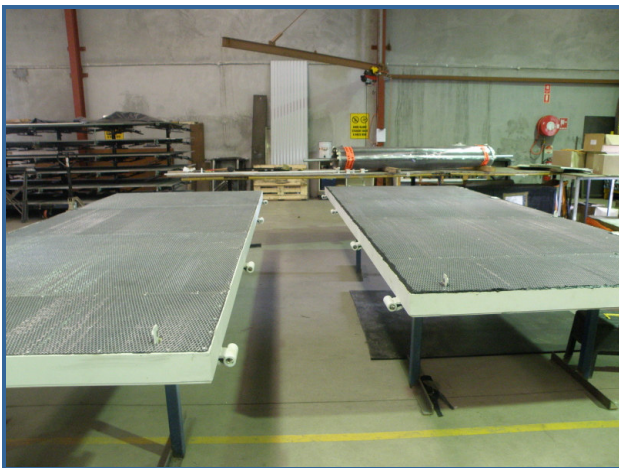
Doors under construction at Hushpak's Adamstown manufacturing plant
